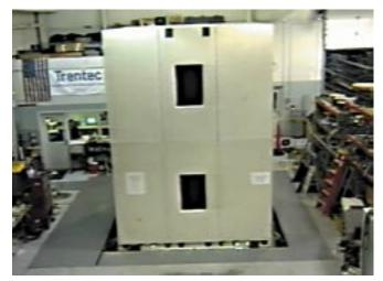
Two-story model ThermaSave panel structure couldn't be damaged by the shake test at the Trentec Lab in Cincinnati, OH.
