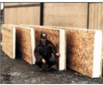
Unlike some structural insulated (SIP) panel systems, the ThermaSave panels vary in size, including both length and thickness, to meet the structural requirements of the building.
